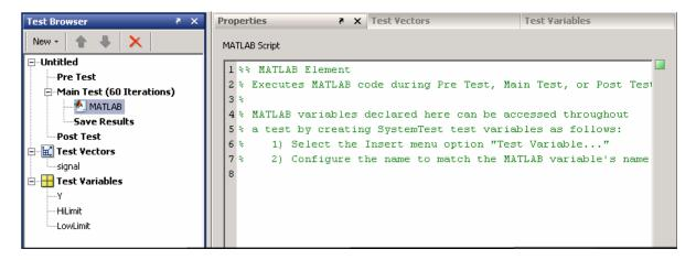
**3** In the **Properties** pane, type the following M-code in the MATLAB Script edit box. This MATLAB code calculates a value for Y that is dependent on the test vector signal.
