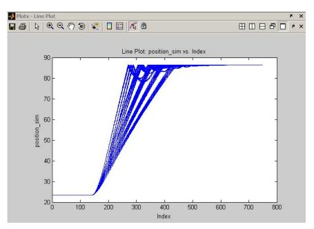
Each line in the plot represents a test iteration. If it appears that there are not as many lines as you had test iterations, it is possible that two or more iterations generated similar enough results that they overlap.
