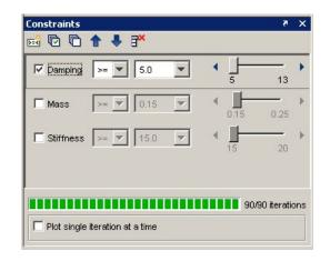
**3** Click the right-pointing arrow at the end of the **Damping** constraint's slider.
