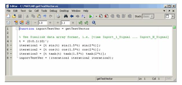
Once this function is saved as GETTESTVECTOR, you can create a SystemTest test vector whose expression is set to GETTESTVECTOR. This will create a 1-by-3 test vector cell array within the SystemTest software, where each entry in the cell array represents the time and signal data for the three Inport blocks. For detailed information on the Simulink data array format, or other formats supported by Simulink Inport blocks, see Importing and Exporting Simulation Data in the Simulink documentation.
