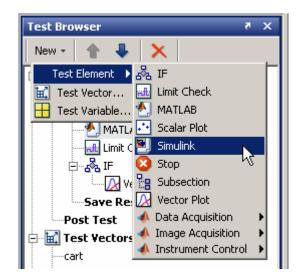
The SystemTest<sup>TM</sup> software adds the Simulink element to the test and opens the Simulink element **Properties** pane.
